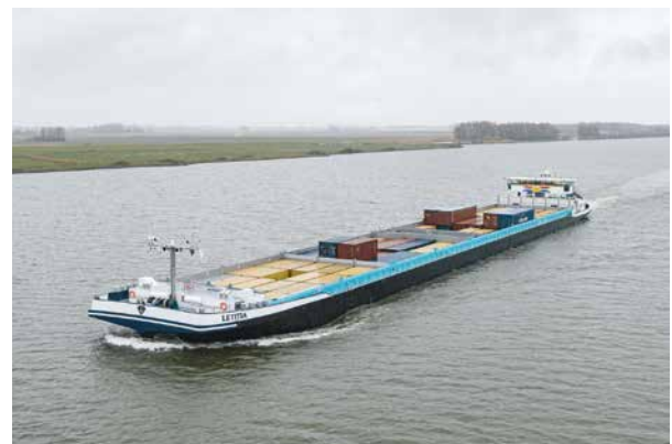
Fig. 4: In the middle of the MS Letitia there are four container areas separated by two partitions, which are capable of holding a total of 16 energy containers for the fuel cells, the batteries and the tank containers [Source: RensenDriessen Shipbuilding, Photo Maritime Filming Group]
