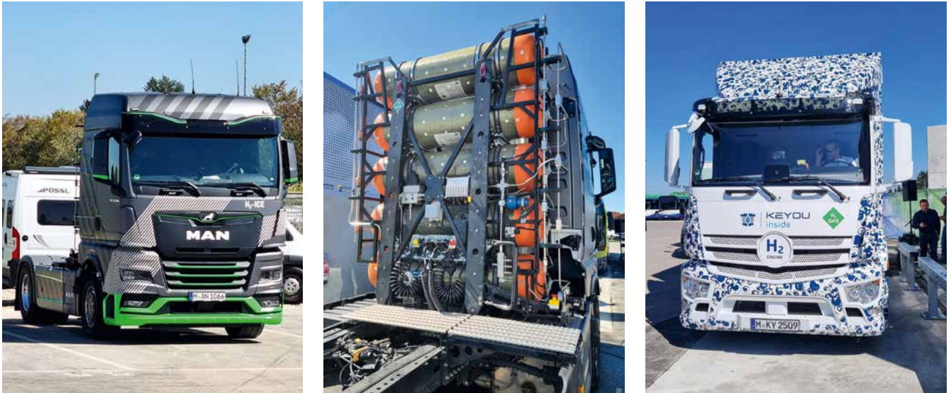
Fig. 4: MAN H 2 -ICE tractor unit with 70 MPa pressure hydrogen-storage module (left) and Keyou H 2 -ICE truck with 35-MPa storage system [Source: R. Wurster]
