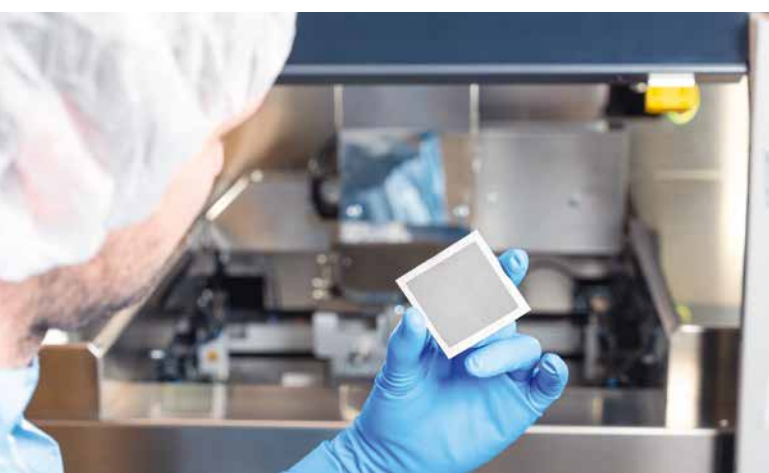
Fig. 6: Fraunhofer ISE has produced a microporous titanium layer on a titanium fiber substrate with the screen printing process, which is supposed to serve as an MPL [Source: Fraunhofer ISE / Joscha Feuerstein]
